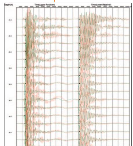
*Example of data created by the PS Logger Probe.*
