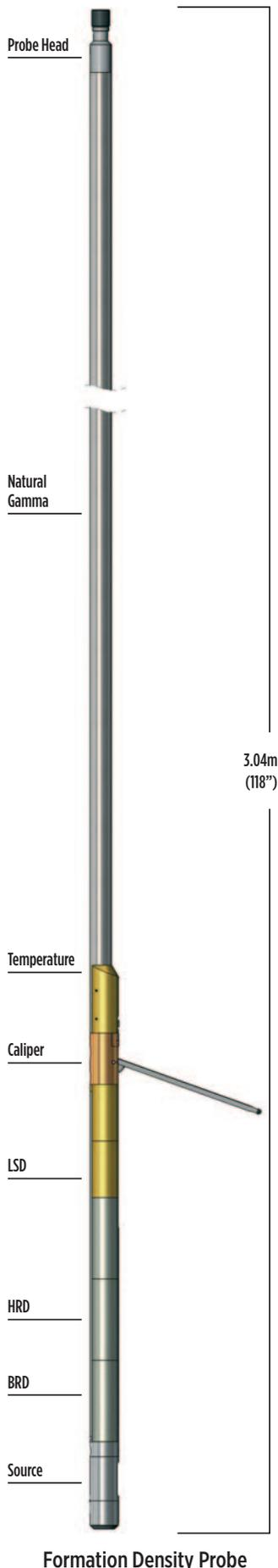
The Formation Density probe uses dual shielded detectors to provide a borehole-compensated density measurement with good bed-boundary resolution.
